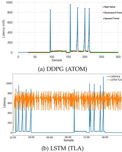
Fig. 8. Performance comparison of ATOM and TLA in terms of latency.
