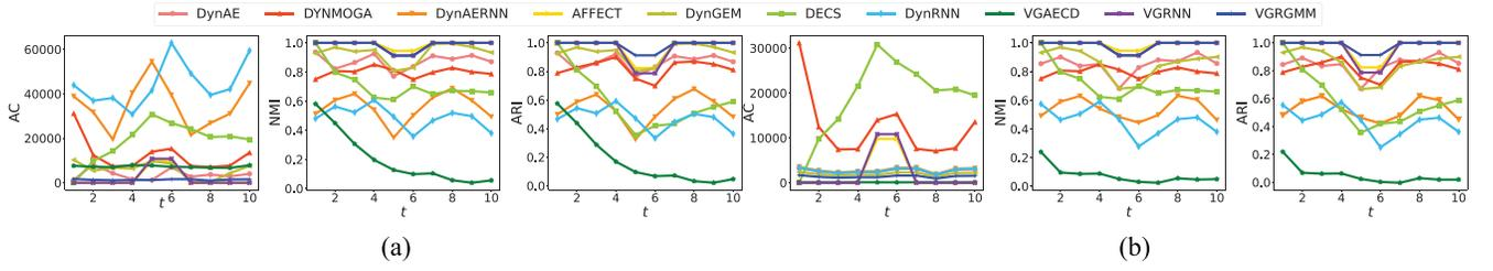
Fig. 2. Experiment results on the two generated dynamic networks with the ground truth. (a) Var dataset. (b) Synth dataset. The performance results are based on the AC, NMI, and ARI, respectively. Each value is computed by the average of ten randomly generated networks with the same parameters.
