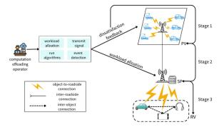
Fig. 1. Overall architecture of our PVEC system.
