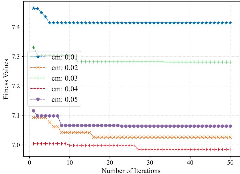
Second, the effects of the mutation probability on GATC are investigated in terms of the obtained optimal values and the response latency. The results are shown in Figs. 6 and 7, respectively. We denote the mutation probability by  $cm$  in the experiments. Similar to the evaluation of crossover probability in the first set of experiments, five values for  $cm$  are investigated. Other parameters are also set to default values
