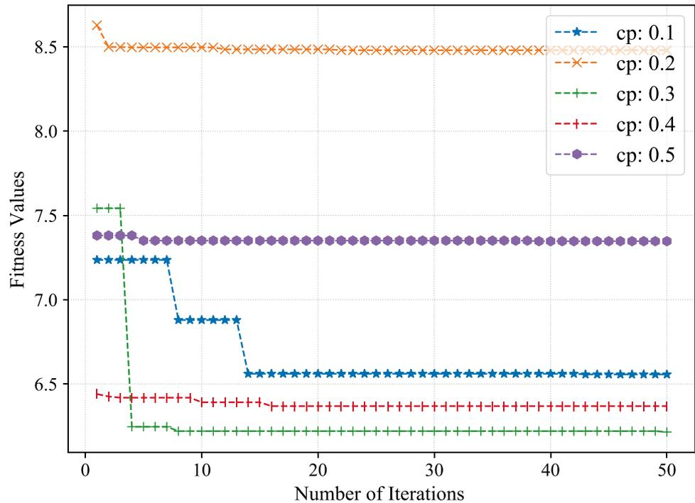
stuck in different locally optimal solutions respectively. We also notice that no matter which case is considered, the obtained fitness values do not change any more when the number of iterations comes to 20. The response times are shown in Fig. 5 when the different crossover probability is considered. The number of iterations is up to 20. This is because the fitness values as shown in Fig. 4 do not change
