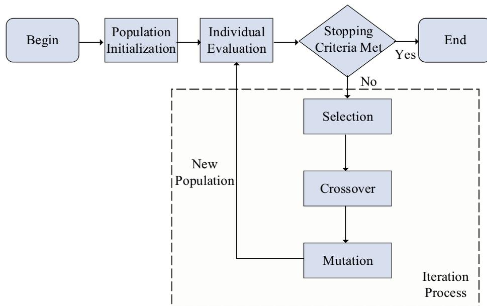
crossover operation is implemented by exchanging the gene segments between two parents. In this paper, we adopt a multiple point crossover to generate the offsprings [23]. Specifically, an example of multiple point crossover operation is depicted in Fig. 2.
